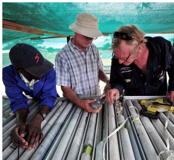
Drill core showing banded copper-bearing schist
