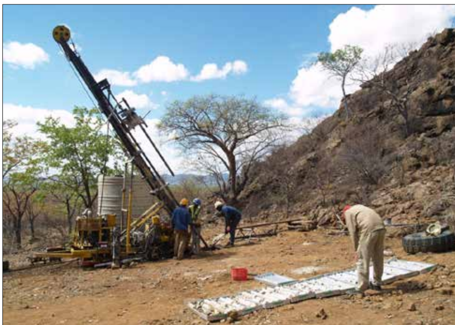
Photo 12. Diamond drilling at Epembe.
