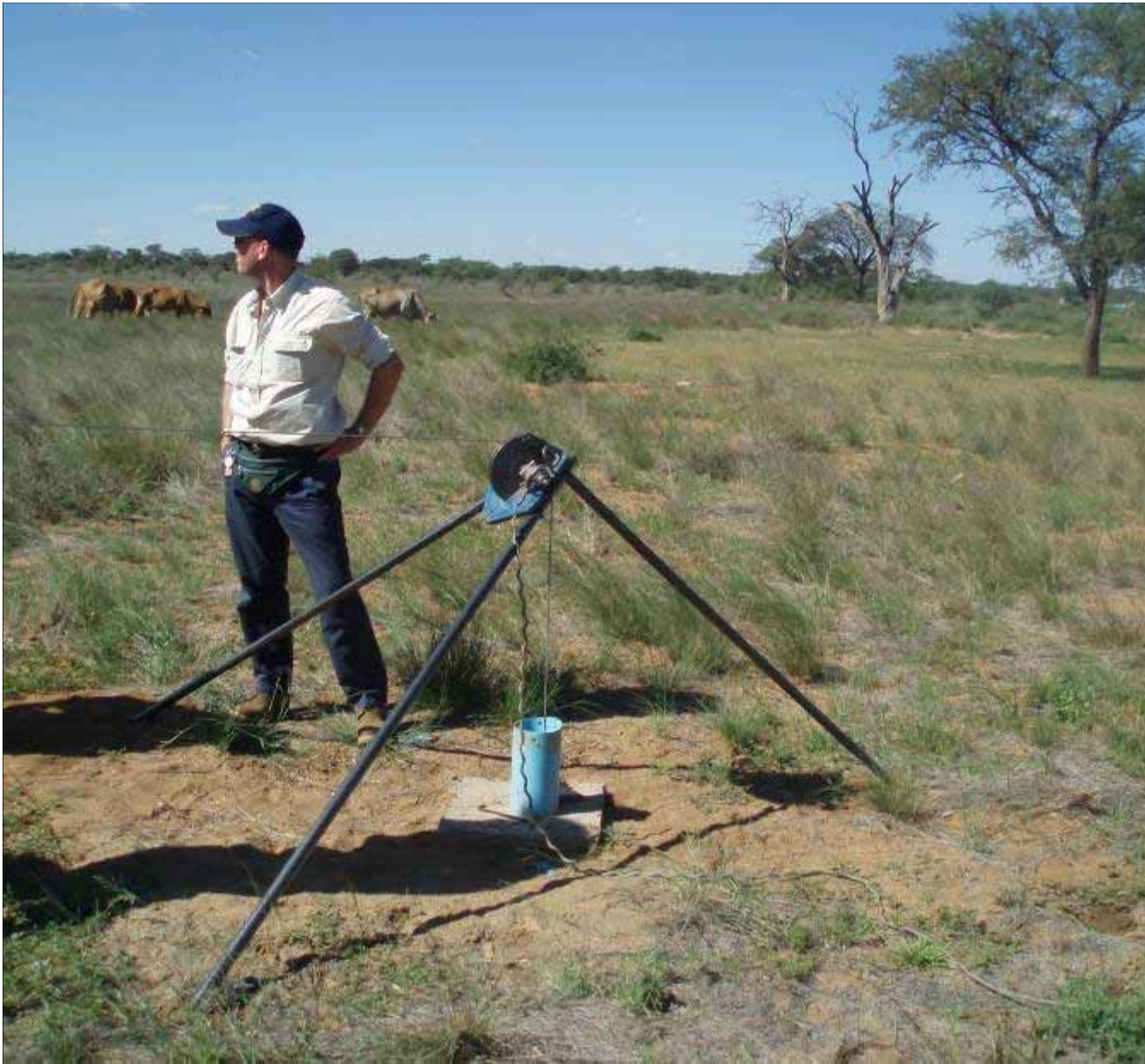
Down-hole photography assists in determining geological structure
