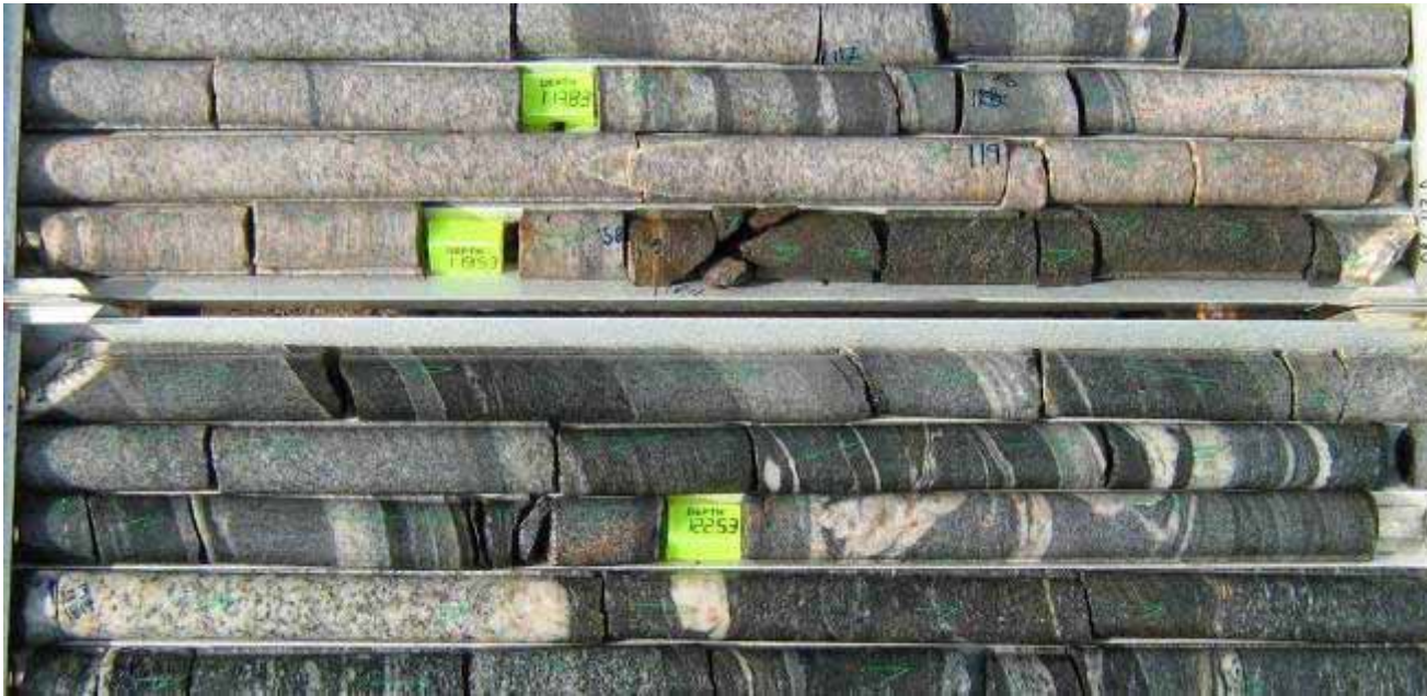
Hangingwall contact – barren gneiss (at top), over-lying mineralised dark banded biotite schist (Hole ORC117)
