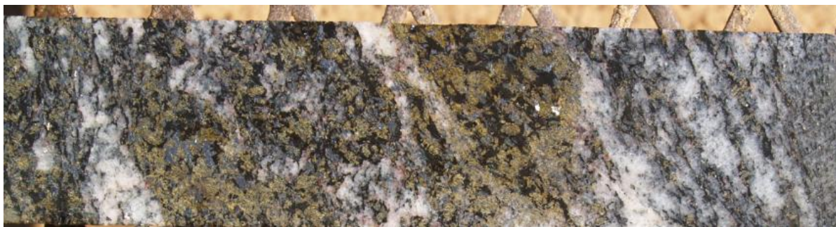
Figure 3. Drill core from a recent drill hole, showing strongly sheared high grade ore with greenish brown epidote and steel-grey chalcocite (core diameter =5cm)
