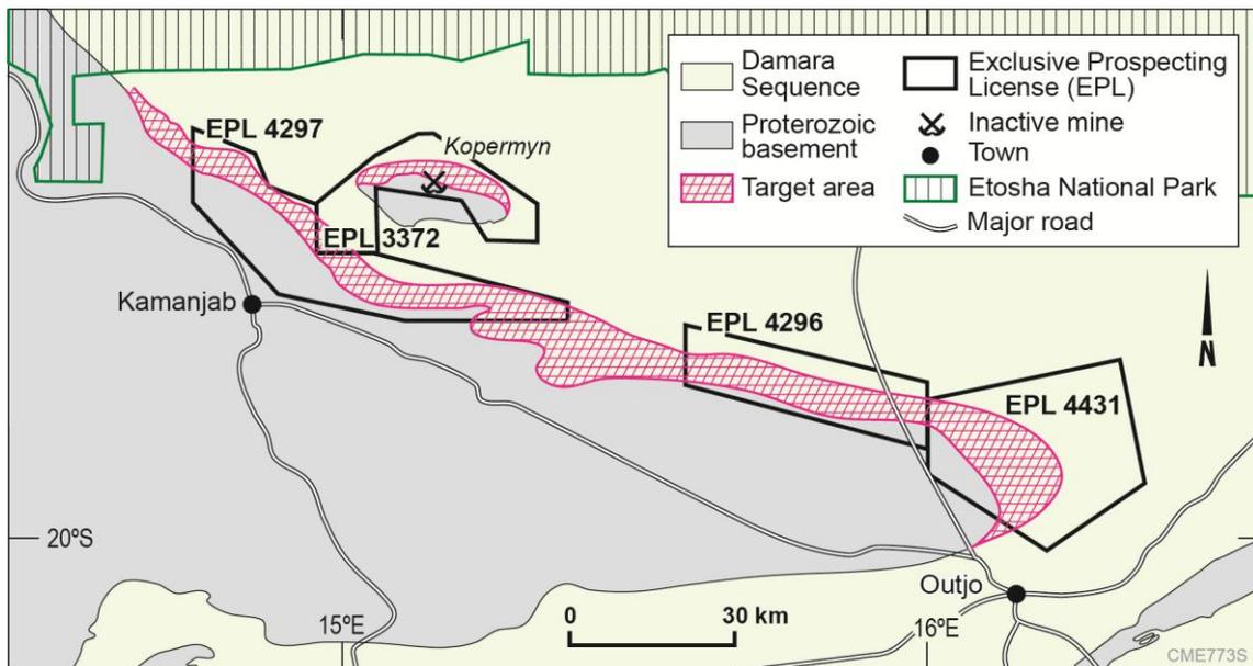
Figure 20. Kamanjab Project: Geological setting and tenements
