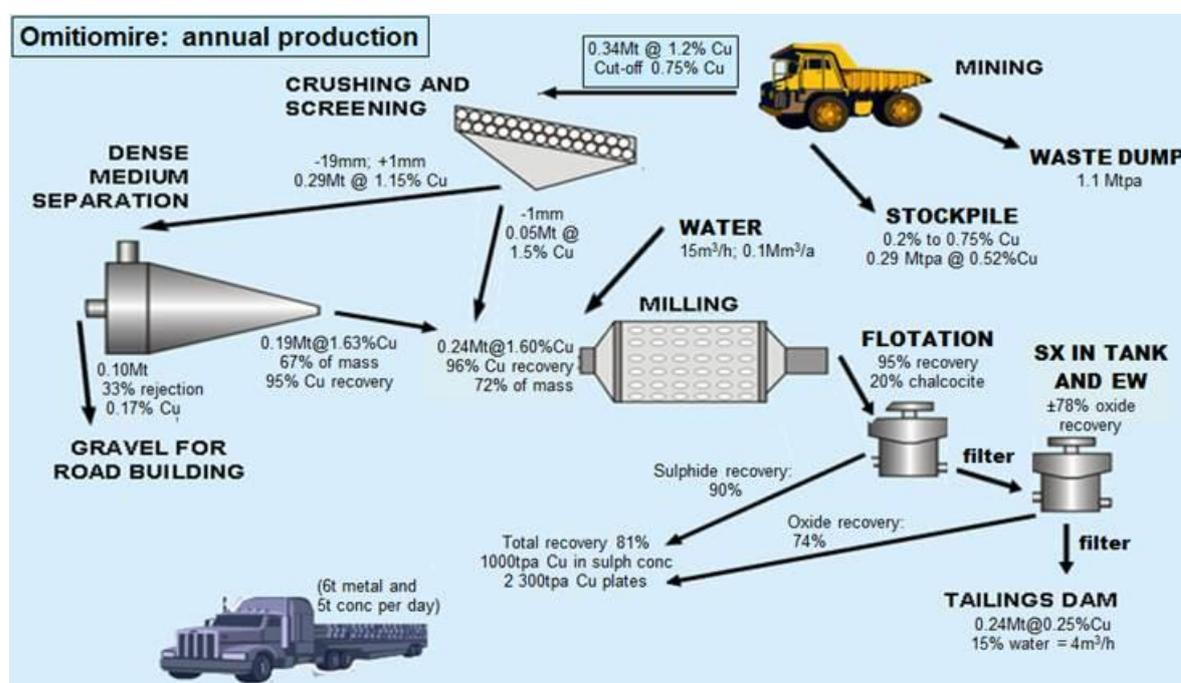
Figure 7. Processing flow sheet envisaged for a Phase 1 oxide copper operation
