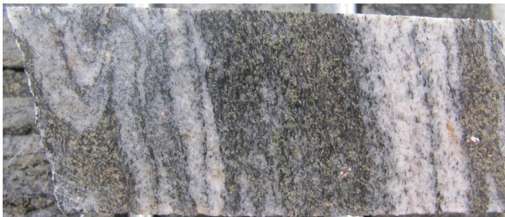
*Photo 1. Recumbent fold in drill core*
