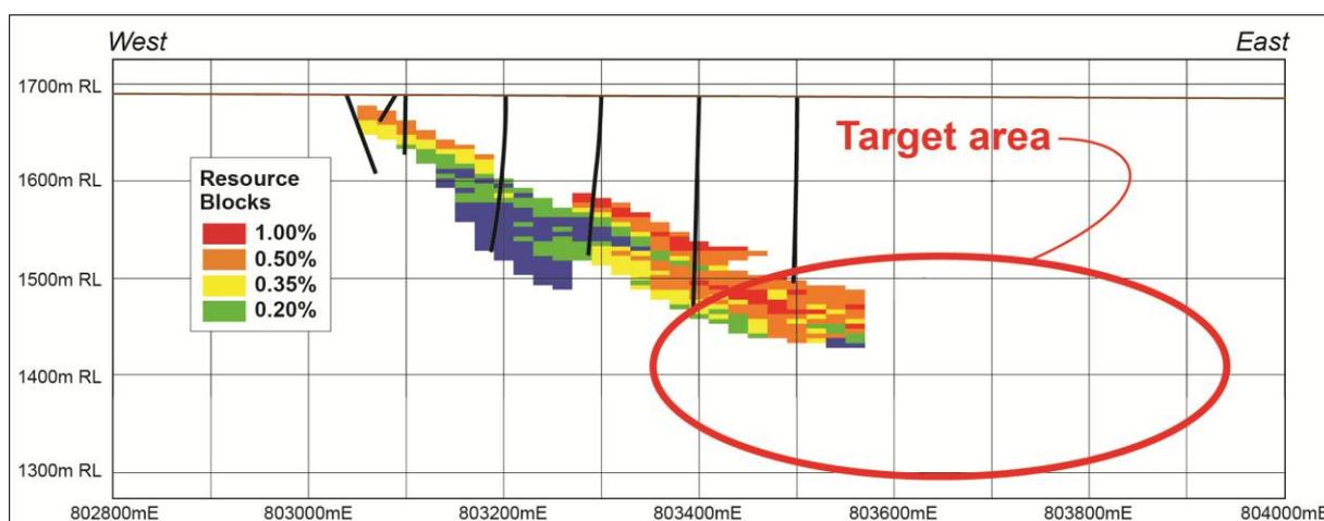
Figure 2. Section 3870 showing resource blocks as at mid-2011 and down-dip target
