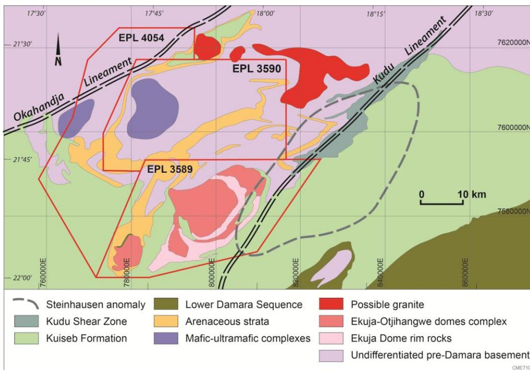
Figure 11. Geological interpretation of the northern portion of the Steinhausen Project area, showing the nappe complex
