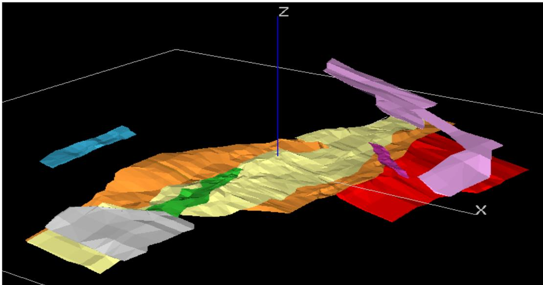
Figure 3. Isometric view of the 2012 resource wireframes. The model identifies eight lenses: A (yellow); B (orange); C (red); Central (green); Kaya (grey); Mamba (blue); Bruce (pink) and Bruce Terrace (purple). Almost half the resource tonnage is within the B Lens
