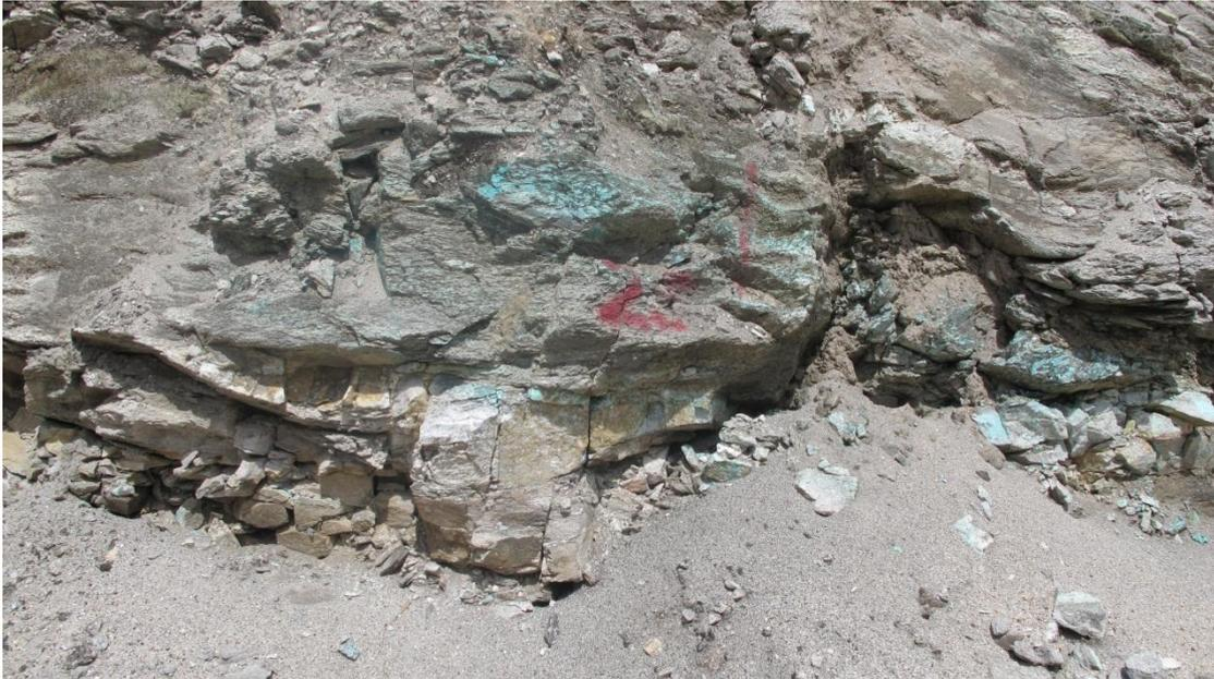
*Photo 2. Oxide copper (blue-green) exposed in the bulk sample pit*
