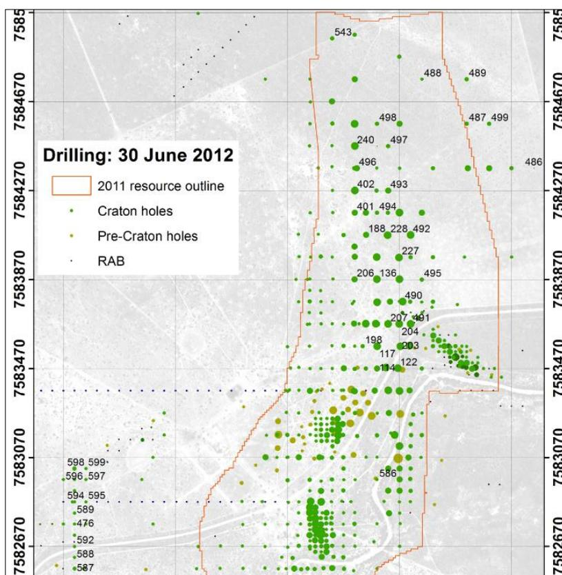
Figure 6. Drill hole plan. Holes completed during 2012 are numbered. Symbol size is proportional to the thickness x grade intersected. The three clusters of closely-spaced holes are the near-surface oxide copper zones. The south-western cluster of holes targeted the Mamba Lens
