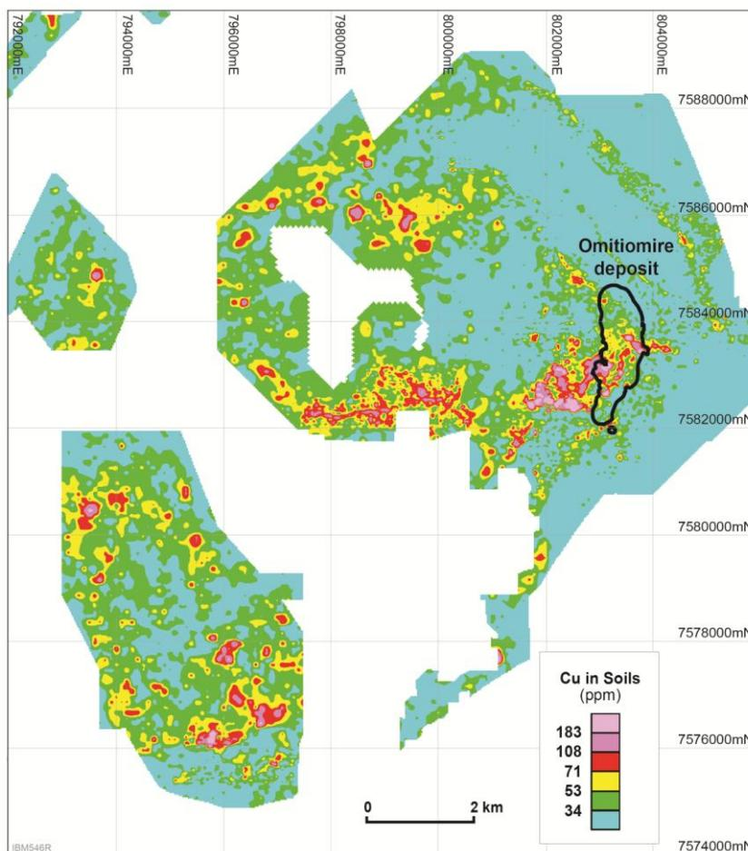
Figure 9. Detailed soil geochemistry of the Ekuja Dome, showing extensive copper anomalies within trucking distance of Omitiomire
